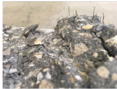
(c) micro steel fibers
