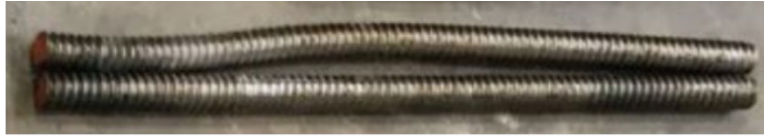
Figure 3.27 Deformation of the dowel bars in SMART Shear Key 3
